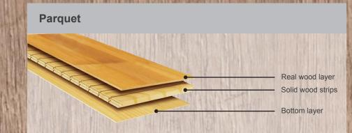
Parquet with two or three layers can be bonded with D3 PVAc dispersions as well as with PUR hot melt adhesives. The dispersions are applied on the full surface of the wood substrate. After drying, the real wood layer is usually applied in the form of different strip geometries and the two layers are pressed. An adhesive bead of PUR hot melt is usually applied on the substrate after which it is joined with the real wood layer in an inline pressing procedure, creating an even bonding result.
